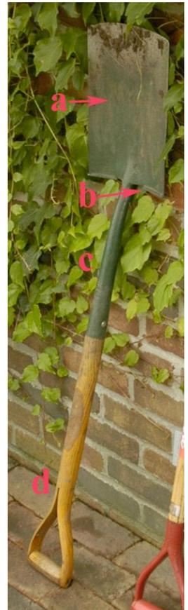
This most durable tool we've ever met has **a drawback -- its weight**. It's made of very durable steel and shaped with an extra long socket (c in these photos) to clad the handle. It's for serious gardeners who use it every day, sometimes for hours at a time and include non-standard uses such as for boulder-levering and root-ball shifting.
