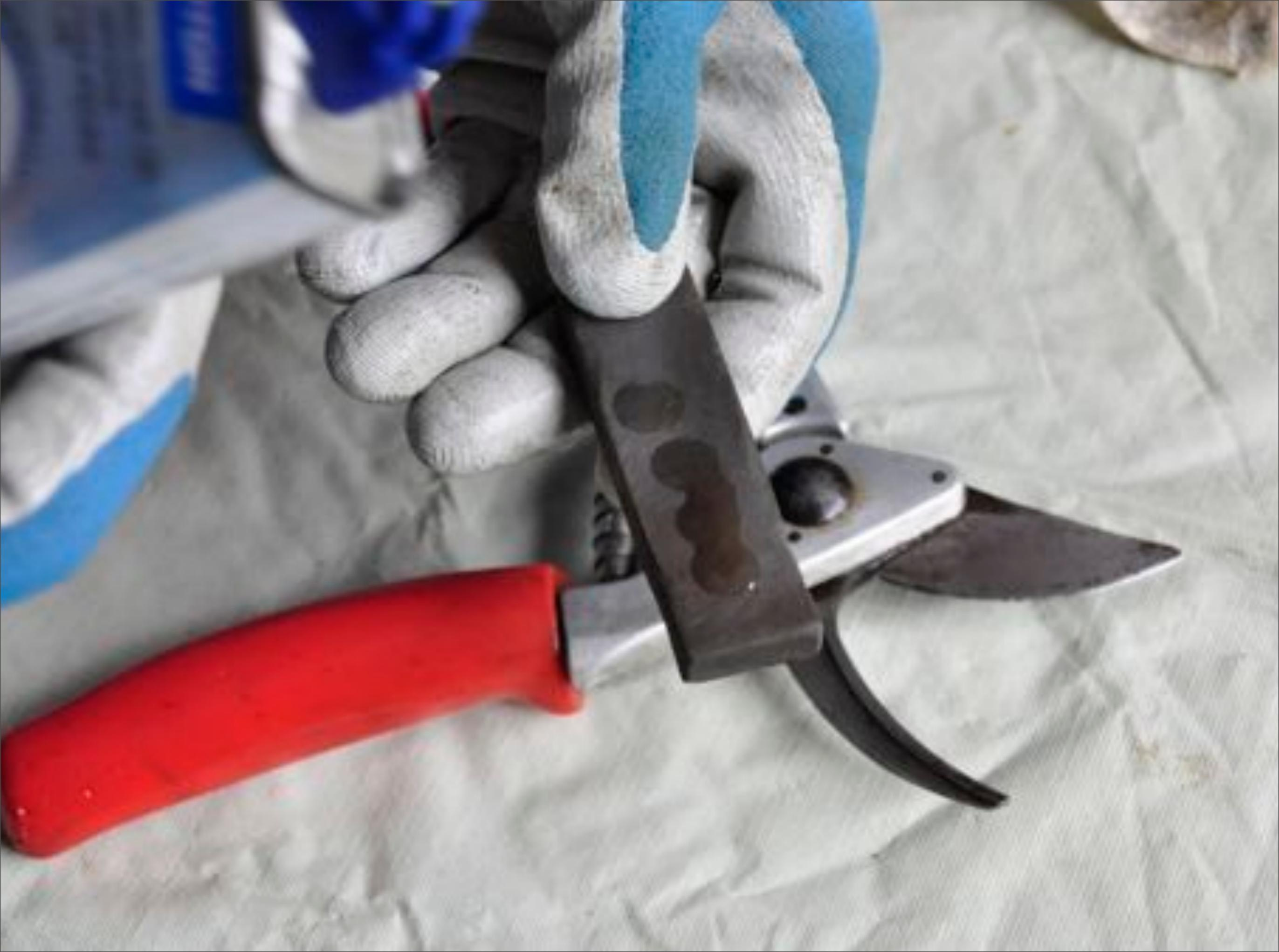
The oil soaks in. Tiny bits of metal that come off as you hone will float away in an oil film.
