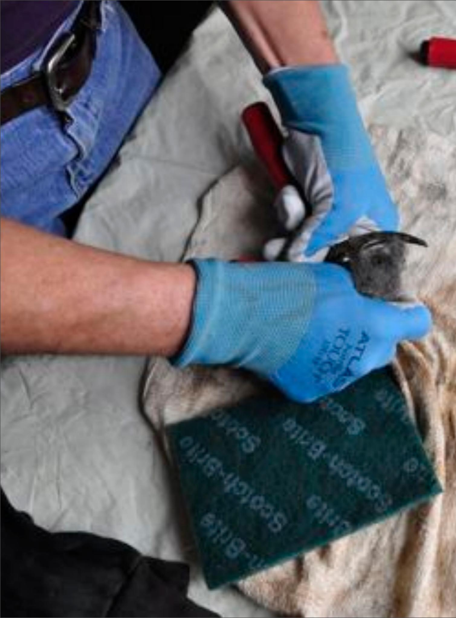
You do NOT want to sharpen a dirty, rusty edge because dirt will scratch the blade. Meanwhile, tiny bits of rust will be dragged out and pressed into the new edge, “seeding” more rust
